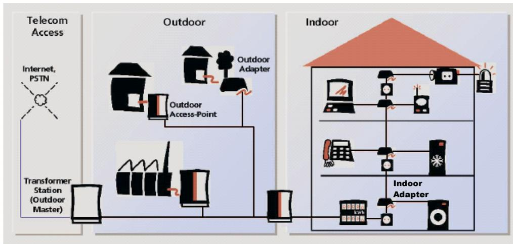
**Figure 2. Complementing outdoor and indoor systems for maximum coverage**
