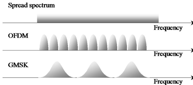
**Figure 1. Modulation techniques for PLC systems**
